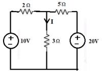
7. a) State and prove Compensation theorem.[5M]b) Verify Tellegen"s theorem for the circuit shown in below figure.[5M]
