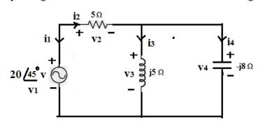
8 .a) State and prove Milliman"s theorem.[5M]b) Verify reciprocity theorem for the network shown in below figure.[5M]
