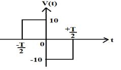
6. a) Find the Trigonometric Fourier series for the waveform shown in figure and sketch the spectrum.
